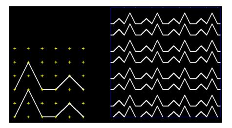
In the next figure, instead, the lines on the right do not end where the lines on the left begin, and a discontinuity is noticed in the repeated pattern forming the hatch.
