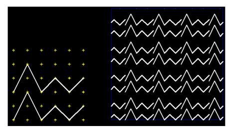
For this reason the preparation of complex sketching require often a definition of the base figure on an little more extensive area than the grid, in the way of moving then the external elements down or left, repeating the operation until all the lines are internal to the grid.
