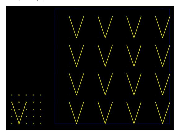
In order for the pattern you draw to be convertible in hatch, it is necessary that the vertices of the lines perfectly match with the points of the grid During the conversion in hatching, the lines with vertices
